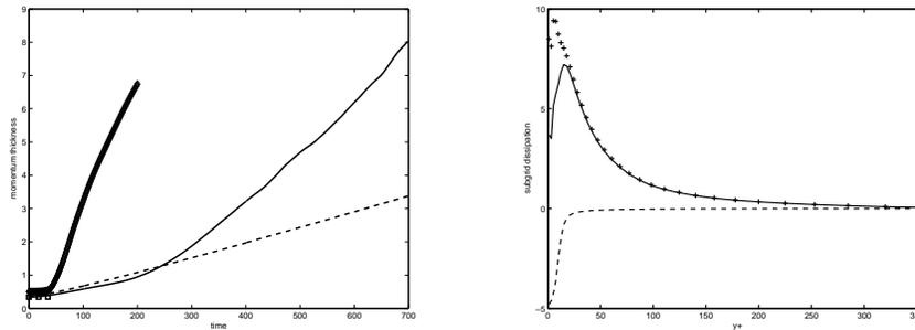
**Fig. 1.** LEFT: Evolution of momentum thickness in supersonic mixing layer at  $M_c = 2.0$  for three subgrid models: Equation (1) (solid), Smagorinsky model (dashed), dynamic model (squares). The reference curve at  $M_c = 0.28$  [1] is also shown (thick curve). RIGHT: subgrid dissipation of adjoint filtered model, Eq. (5), in LES of channel flow (solid), decomposed into forward scatter ('+') and backscatter (dashed).
